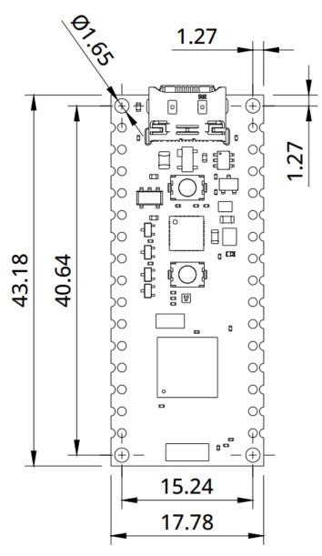
The Nano Matter has four 1.65 mm drilled mounting holes for mechanical fixing.
