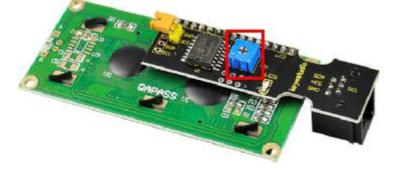
Note: rotate the blue potentiometer(screwdriver is not included) to adjust the brightness of the 1602 LCD.
